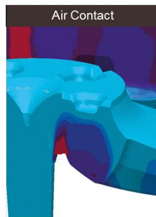
MAGMASOFT® results for mold filling and analysis of potential casting defects such as cold shuts or oxide inclusions
