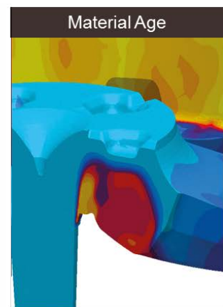
MAGMASOFT® results for mold filling and analysis of potential casting defects such as cold shuts or oxide inclusions
